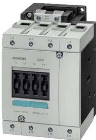
CONTACTOR, AC-1 110 A, AC 120 V 60 HZ 4-POLE, SIZE S3, SCREW CONNECTION
