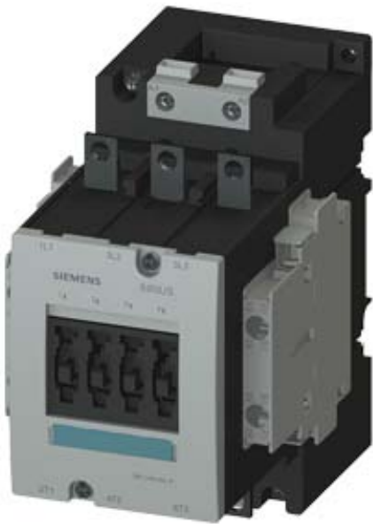
CONTACTOR 1-PH, 140A/400V 480 V AC, 60 HZ AUX. CONTACTS 2N + 2NC LATERAL 3-POLE, SIZE S3 BAR CONNECTIONS
