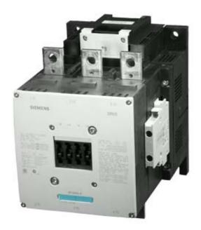
CONTACTOR, 690A/AC-1 AC(40...60HZ)/DC OPERATION UC 440-480V AUXILIARY CONTACTS 2NO+2NC 3-POLE, SIZE S12 BAR CONNECTIONS CONVENT. OPERATING MECHANISM
