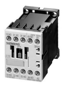
CONTACTOR 3-PH 5.5KW/400 V, AC-1 22 A, 110 V DC 4-POLE, 2 NO + 2 NC, SIZE S00, SCREW CONNECTION
