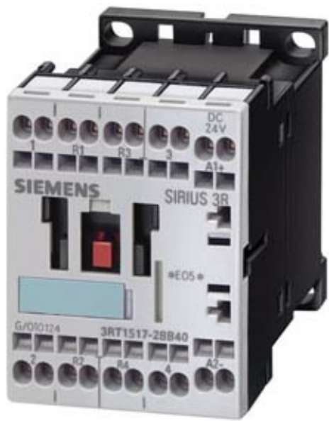
CONTACTOR, AC-3 5.5KW/400V, AC-1 22A, AC 48V, 50HZ, 4-POLE, 2 NO + 2 NC, SIZE S00, CAGE CLAMP CONNECTION
