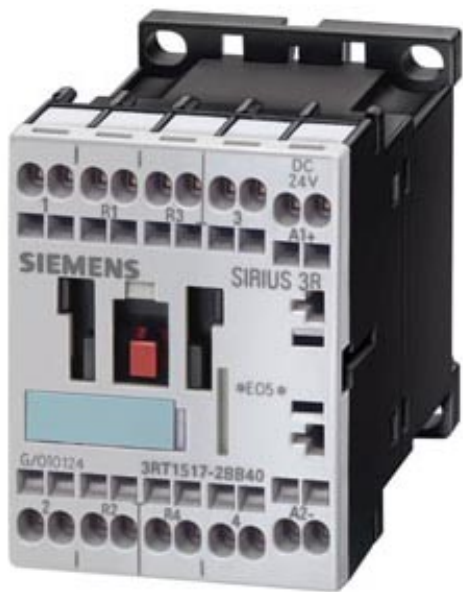
CONTACTOR, AC-3 5.5KW/400 V, AC-1 22A, DC 48 V, 4-POLE, 2 NO + 2 NC, SIZE S00, CAGE-CLAMP CONNECTION
