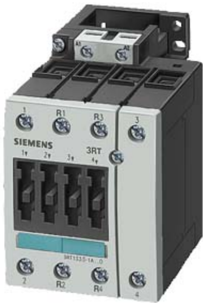
CONTACTOR, AC-3 18.5 KW,400V, AC 24 V, 50/60 HZ 4-POLE, 2 NO + 2 NC, SIZE S2, SCREW CONNECTION
