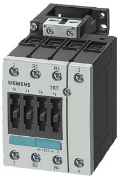
CONTACTOR 3-PH 18.5 KW,400V, 42 V AC, 50 HZ 4-POLE, 2NO + 2NC, SIZE S2, SCREW CONNECTION
