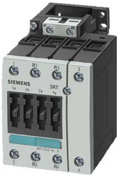
CONTACTOR, AC-3 18.5 KW,400V, AC 42V, 50/60HZ 4-POLE, 2 NO + 2 NC, SIZE S2, SCREW CONNECTION
