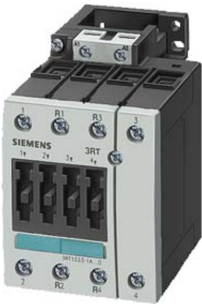
CONTACTOR, AC-3 18.5 KW,400V, AC 110V, 50 HZ 4-POLE, 2 NO + 2 NC, SIZE S2, SCREW CONNECTION
