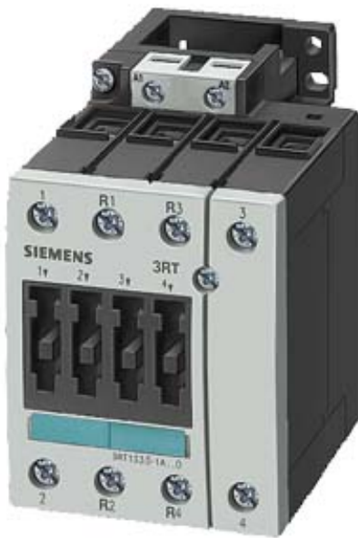
CONTACTOR, AC-3 18.5 KW,400V, AC 24 V, 50 HZ 4-POLE, 2 NO + 2 NC, SIZE S2, SCREW CONNECTION
