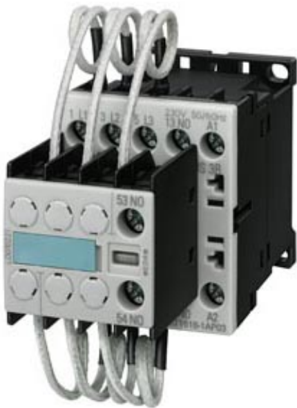
CAPACITOR SW. CONTACTOR, AC-6, 12.5KVAR/400V, AC 100V 50/60HZ/ AC 110V 60HZ, 3-POLE, SIZE S00
