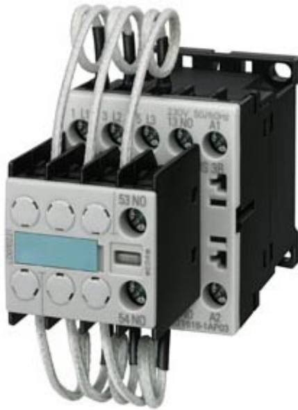
CAPACITOR SW. CONTACTOR, AC-6, 12.5KVAR/400V, AC 220V 50HZ/ AC 240V 60HZ, 3-POLE, SIZE S00
