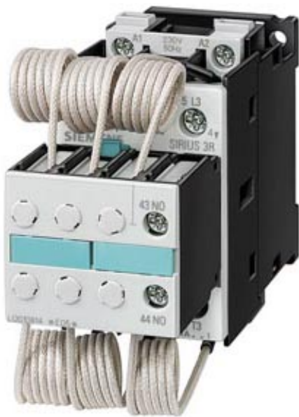
CAPACITOR SW. CONTACTOR, AC-6, 25KVAR/400V, 230V, 50/60HZ, 3-POLE, SIZE S0
