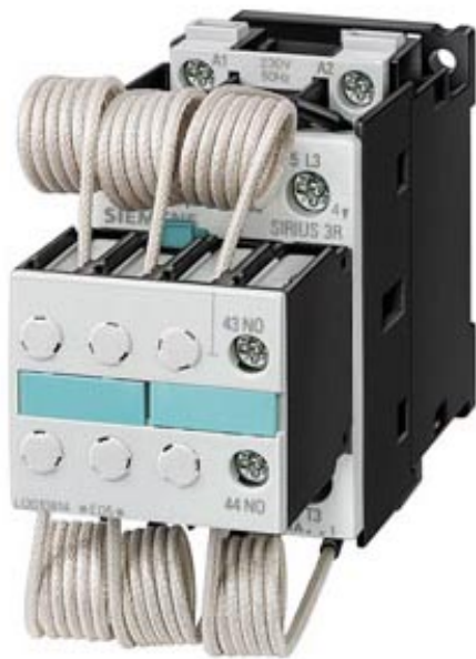
CAPACITOR SW. CONTACTOR, AC-6, 25KVAR/400V, 220V, 50/60HZ, 3-POLE, SIZE S0
