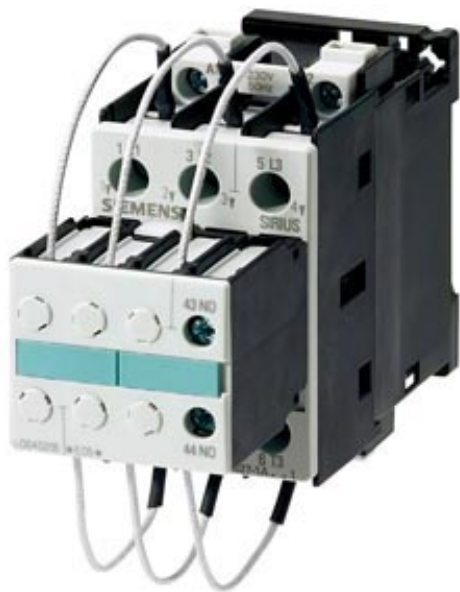
CAPACITOR SW. CONTACTOR, AC-6, 25 KVAR/400V, 400V, 50HZ, 3-POLE, SIZE S0
