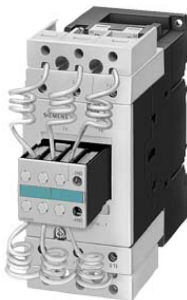
CAPACITOR SW. CONTACTOR, AC-6, 50KVAR/400V, 24V, 50/60HZ, 3-POLE, SIZE S3
