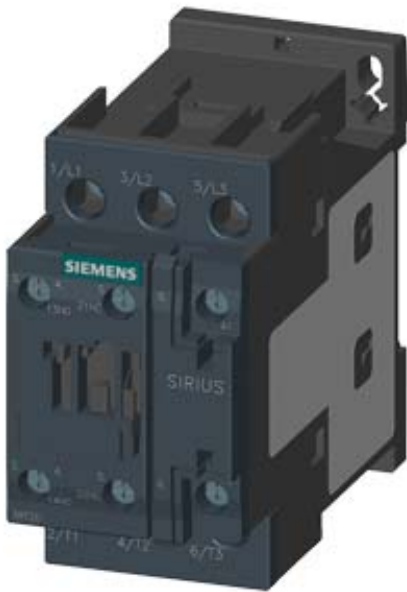
CONTACTOR, AC-3, 4KW/400V, 1NO+1NC, AC 220V 50/60HZ, 3-POLE, SZ S0 SCREW TERMINAL
