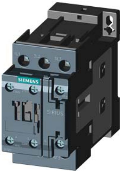
CONTACTOR, AC-3, 5.5KW/400V, 1NO+1NC, DC 110V, 3-POLE, SZ S0 SCREW TERMINAL
