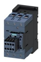
Contactor, AC-3, 55 kW/400 V 2 NO+2 NC, 110 V AC 50 Hz 3-pole, 3 NO, Size S3 Screw terminal
