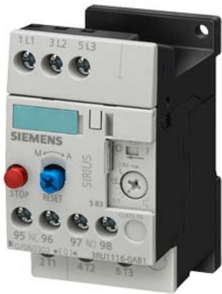
OVERLOAD RELAY, 1.1...1.6 A, 1NO+1NC, SIZE S00, CLASS 10, FOR INDIVID. MOUNTING
