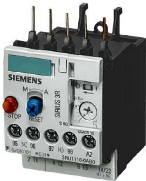
OVERLOAD RELAY, 7...10 A, 1NO+1NC, SIZE S00, CLASS 10, FOR CONTACTOR MOUNTING
