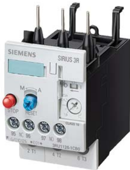
OVERLOAD RELAY, 2.2...3.2 A, 1NO+1NC, SIZE S0, CLASS 10, FOR CONTACTOR MOUNTING
