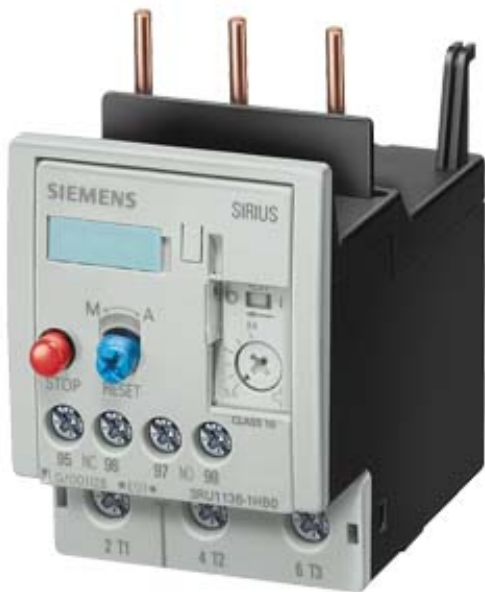
OVERLOAD RELAY, 7...10 A, 1NO+1NC, SIZE S2, CLASS 10, FOR CONTACTOR MOUNTING
