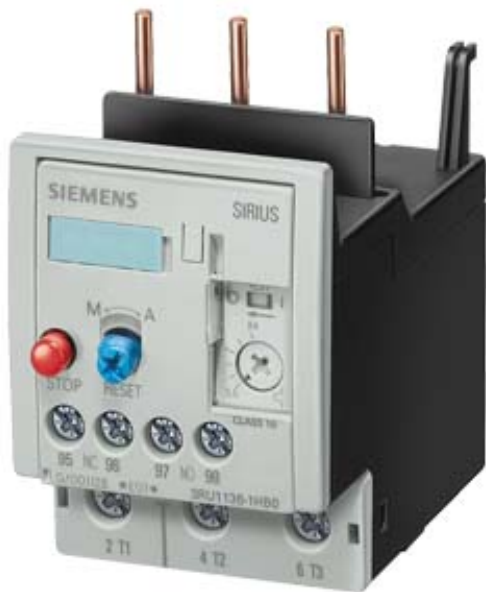
OVERLOAD RELAY, 18...25 A, 1NO+1NC, SIZE S2, CLASS 10, FOR CONTACTOR MOUNTING
