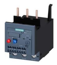
Overload relay 54...65 A Thermal For motor protection Size S2, Class 10 Contactor mounting Main circuit: Screw Auxiliary circuit: spring-type terminal Manual-Automatic-Reset
