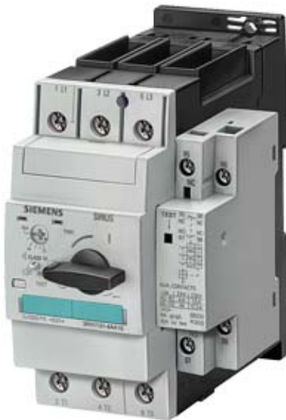
CIRCUIT-BREAKER, SIZE S2, FOR MOTOR PROTECTION, CLASS 10, WITH OVERLOAD RELAY FUNCTION A REL. 32A, M REL- 416A, SCREW CONNECTION, STANDARD BREAKING CAPACITY
