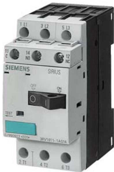
CIRCUIT-BREAKER, A-RELEASE 0.2 A N-RELEASE 1.2 A, SIZE S00, FUSE MONITORING, SCREW CONNECTION
