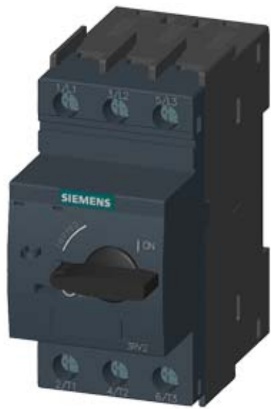
CIRCUIT-BREAKER SZ S0, FOR STARTER COMBINATION, RATED CURRENT 4A, N-REL. 52A SCREW CONNECTION, STANDARD SW. CAPACITY
