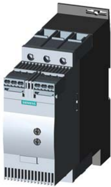
SIRIUS SOFT STARTER, SIZE S2, 63A, 30KW/400V, 40 DEGREES, 200-480V AC, 110-230V AC/DC, SPRING-LOADED TERMINALS
