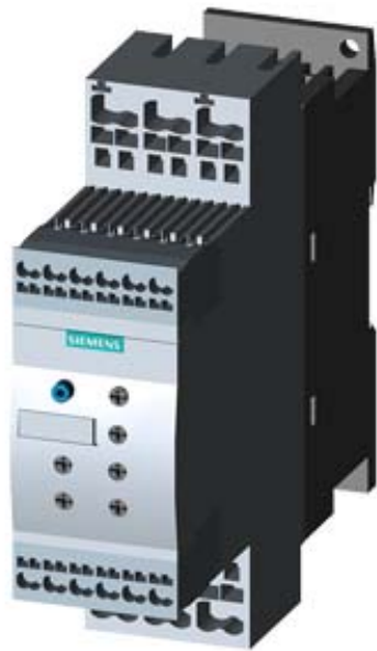
SIRIUS SOFT STARTER, S0, 25A, 11KW/400V, 40 DEGR., AC 200-480V, AC/DC 24V, SPRING-LOADED TERMINALS
