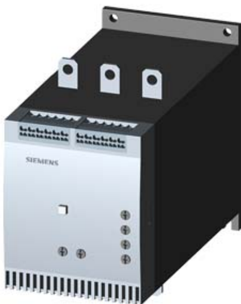
SIRIUS SOFT STARTER, S6, 117 A, 75 HP/460 V, 50 DEG., 200-460 V AC, 115 V AC, CAGE CLAMP TERMINALS
