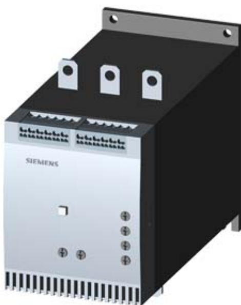
SIRIUS SOFT STARTER, S6, 134 A, 75 KW/400 V, 40 DEG., 200-460 V AC, 230 V AC, CAGE CLAMP TERMINALS
