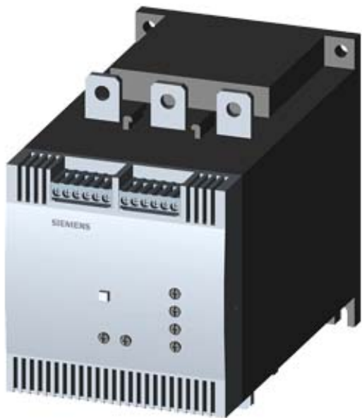
SIRIUS SOFT STARTER, S12, 205 A, 150 HP/460 V, 50 DEG., 200-460 V AC, 115 V AC, SCREW TERMINALS
