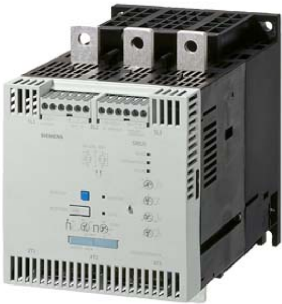
SIRIUS SOFT STARTER, S12, 432 A, 315 KW/500 V, 40 DEG., 400-600 V AC, 230 V AC, SCREW TERMINALS
