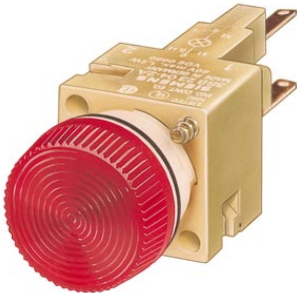
ILLUMINATED PUSHBUTTON, 16MM, ROUND, PLASTIC, RED, BUTTON, RAISED, 1NC, LAMPHOLDER W2 X 4.6D, WITHOUT LAMP
