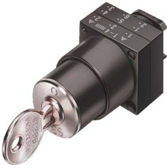
22MM PLASTIC ROUND ACTUATOR: CES KEY- OPER.SWITCH WITH 2 KEYS 3 SWITCH POSITIONS I-O-II LATCHING LOCK NO SSG 10,REMOVAL POS.0+I WITH HOLDER
