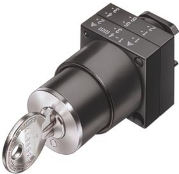
22MM PLASTIC ROUND ACTUATOR: IKON KEY- OPER.SWITCH W. 2 KEYS 3 SWITCH POSITIONS I-O-II LATCHING LOCK NO 360012K1,REMOVAL POS. O WITH HOLDER
