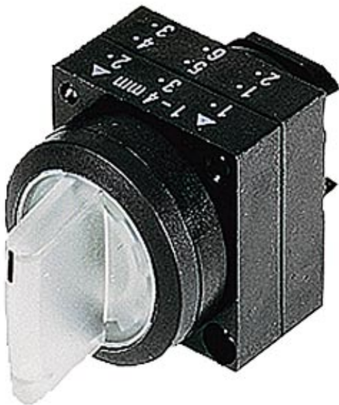
22MM PLASTIC ROUND ACTUATOR: SELECTOR SWITCH RIGHT LATCH.,LE.MOMEN.CONT.TYPE 3 SWITCH POSITIONS I-O-II ILLUMINATED INCL. HOLDER FOR 3 ELEMENTS WITH HOLDER GREEN
