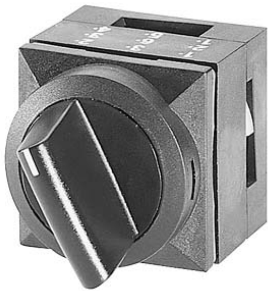
26X26MM PLASTIC SQUARE ACTUATOR: SELECTOR SWITCH LEFT LATCH.,RI.MOMEN.CONT.TYPE 3 SWITCH POSITIONS I-O-II NON-ILLUMINATED WITH HOLDER RED
