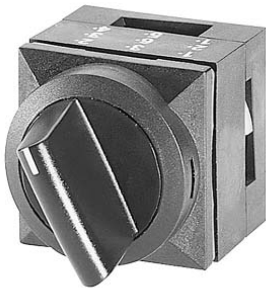
26X26MM PLASTIC SQUARE ACTUATOR: SELECTOR SWITCH LEFT MOMEN.,RI.LATCH.CONT.TYPE 3 SWITCH POSITIONS I-O-II NON-ILLUMINATED WITH HOLDER BLACK
