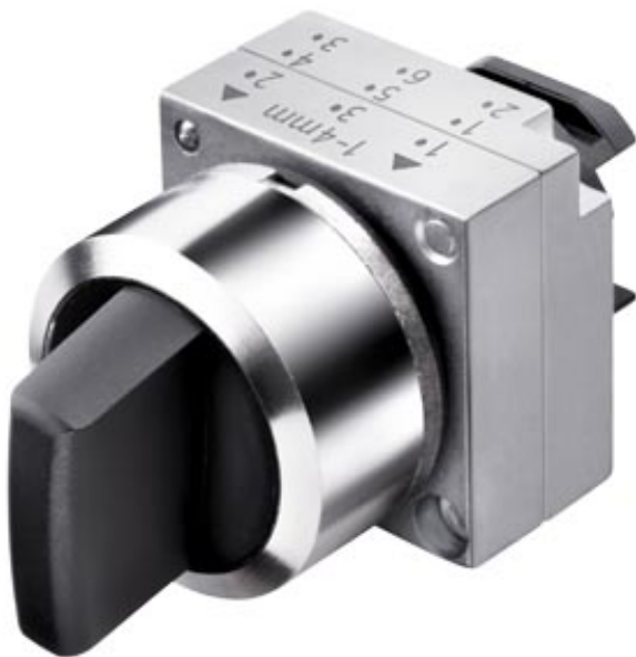
22MM METAL ROUND ACTUATOR: SELECTOR SWITCH HEAVY DUTY RIGHT LATCH.,LE.MOMEN.CONT.TYPE 3 SWITCH POSITIONS I-O-II NON-ILLUMINATED WITH HOLDER BLACK SOLVENT-RESISTANT
