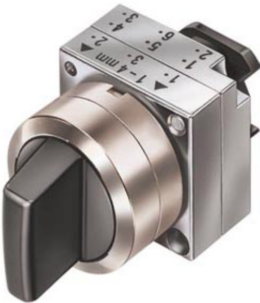
22MM METAL ROUND ACTUATOR: SELECTOR SWITCH LONG HANDLE MOMENTARY CONTACT TYPE 3 SWITCH POSITIONS I-O-II NON-ILLUMINATED WITH HOLDER GREEN
