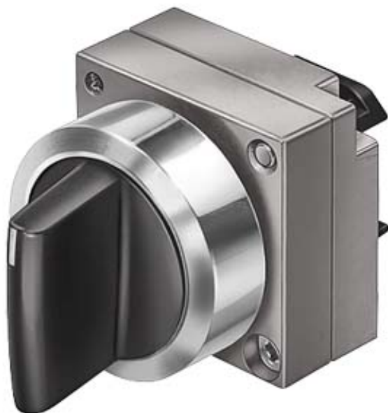
22MM METAL ROUND ACTUATOR: SELECTOR SWITCH LATCHING 2 SWITCH POSITIONS O-I ILLUMINATED WITH HOLDER AMBER
