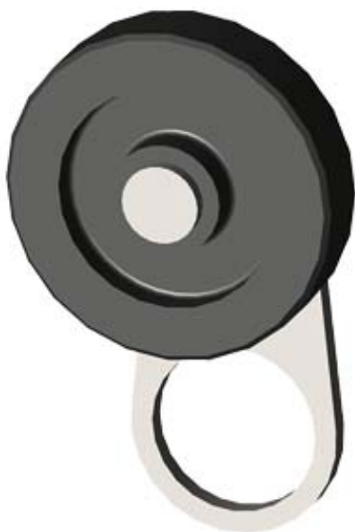
TWIST LEVER FOR POSITION SWITCH 3SE51 METAL LEVER, 27MM LONG,STEP 9MM, W. PLASTIC ROLLER 30MM
