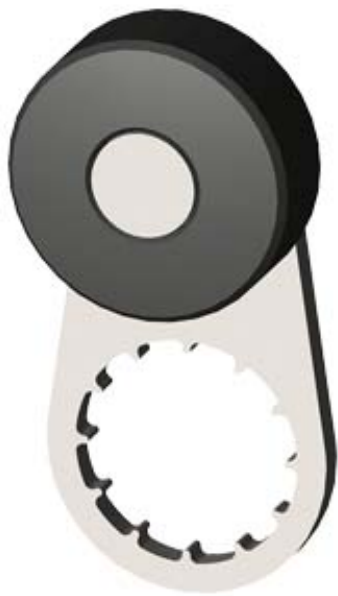
TWIST LEVER FOR POSITION SWITCH 3SE52 STAINLESS STEEL LEVER 21MM LONG PLASTIC ROLLER 19MM FOR ACTUATOR HEAD ACC. TO EN 50047
