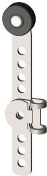
LENGTH-ADJUSTABLE TWIST LEVER FOR POSITION SWITCH 3SE51/52 METAL LEVER 100MM LONG, POSITIVE FIT (HOLE PITCH) PLASTIC ROLLER 19MM
