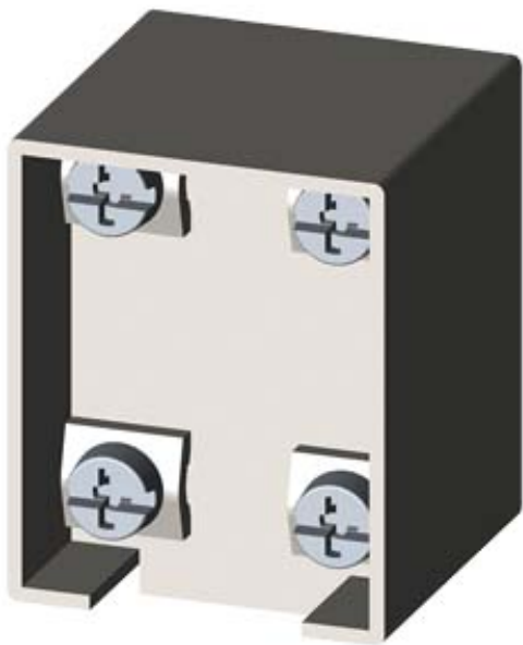
CONTACT BLOCK FOR POSITION SWITCH 3SE51/52 1NO/1NC SNAP-ACTION CONTACT, 2X2MM CONTACT GAP
