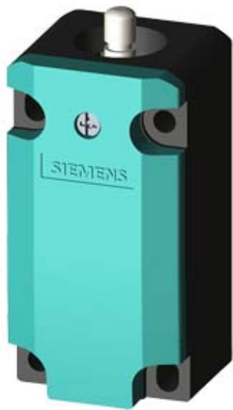
BASIC SWITCH FOR POSITION SWITCH 3SE51, METAL ENCLOSURE, TO EN50041 1X(M20X1.5) 1NO/1NC SLOW-ACTION CONTACTS W/O ACTUATOR HEAD
