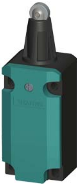
SIRIUS POSITION SWITCH METAL HOUSING 40MM TO EN50041 DEVICE CONNECTION 1X (M20X1,5) 1NO/ 1NC SNAP-ACTION CONTACTS ROLLER PLUNGER W. STAINL. STEEL ROLLER 13MM
